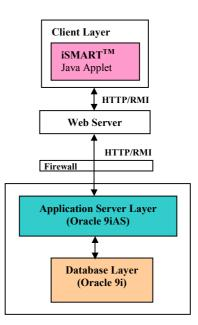
Figure 1. The iSMART<sup>TM</sup> architecture components.
