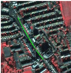
Figure 10. Example of Positioning and radiometric accuracy of IKONOS Precision by k-GPS tracks
