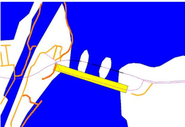
Figure 6: Example of problems produced by scale differences between two vector maps (courtesy Jean Brodeur, NRCan).
