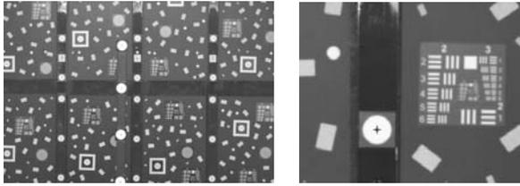
Fig. 5: Sample image of the calibration target (left) and the result of an automated detection of one point target (right)
