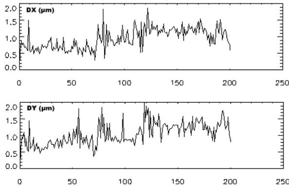
Fig. 6: Deviation of measured image coordinates of 200 target points in the set of 84 images in x-direction (top) and y-direction (bottom)
