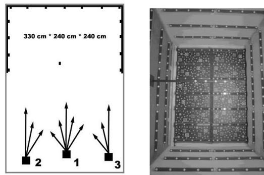
Fig. 4: Three Camera positions are established (left) and a set of 84 images is produced by rotating and tilting (right) the camera.
