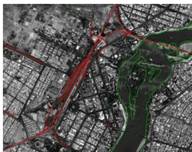
Figure 5. Overlay of vectors on the orthorectified image.
