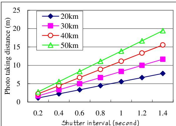
Figure 3-3: Shutter interval and photo taking distance of camera sensor
