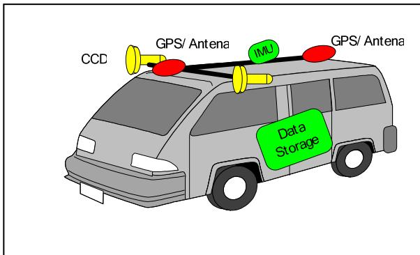
Figure 5-2: Image of measuring vehicle
