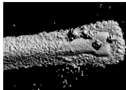
Figure 4. Hillshade of laser data grid of a typical groyne with some bushes on it (grid cell size: 20 x 20 cm 2 ).
