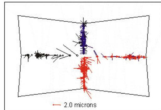
Figure 6. Example of the residuals of the internal bundle orientation,  $\sigma_0 = 0.82\mu\text{m}$  based on 999 observations
