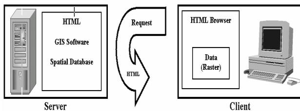
Figure 1. Thin Client Architecture
