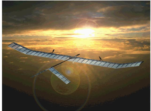
Figure 1. Artist impression of the Zephyr, a light weight HALE UAV
