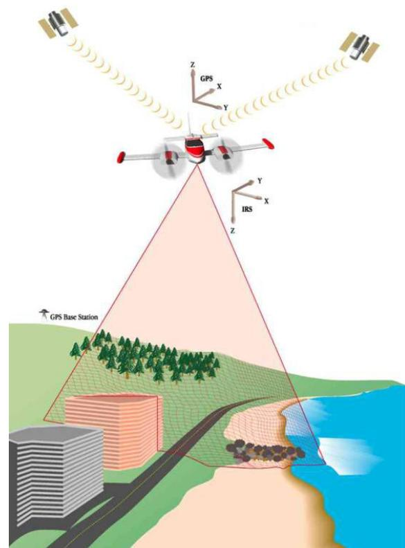
Figure 1. Operating principle of LIDAR system
