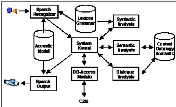
Figure 3. System configuration of HLT [2].
