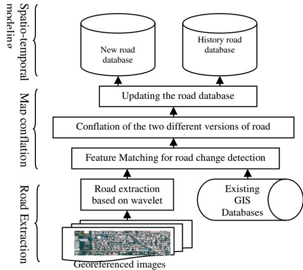
**Figure 1** The proposed framework for an operational road database updating system
