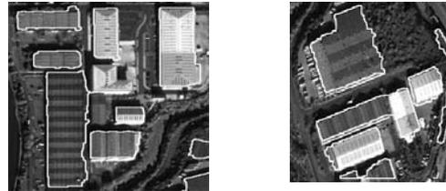
Figure 4. The first refinement result of building ROI by clustering scheme (missing Lidar points over some “hidden” buildings results in no identification.)
