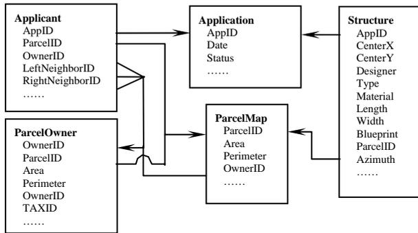
Figure 5. Logical Data Model of the Coastal Structure Permit System.
