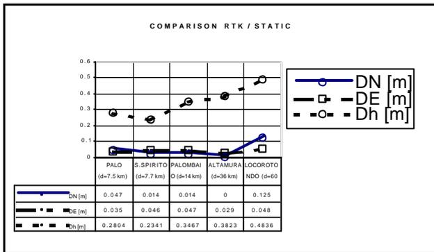
Fig 7 Comparison between DGPS-RTK data gotten with Leica SR530 and known coordinates.
