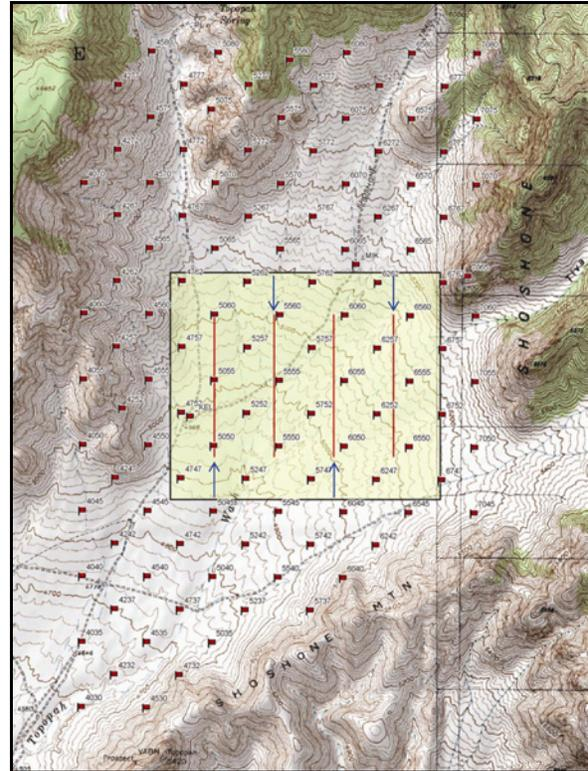
Figure 8. Flight plan with four strips of 25 images to be tested. Image scale will be 1:18,000.
