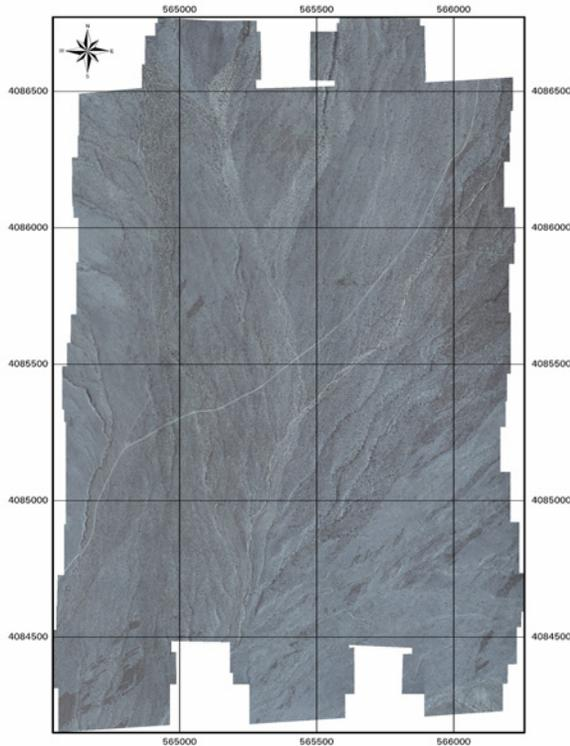
Figure 7. Mosaicked orthophoto map processed from 65 images using a DEM from 60 models.
