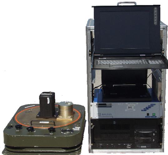
Figure 5 Integrated RTPMS consisting of a DFC, POS, PAV-20 mount and a computer with the OPPP software.
