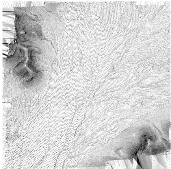
Figure 6. Contour map generated from a block of three strips with 15 images. Contour interval is 1 meter.
