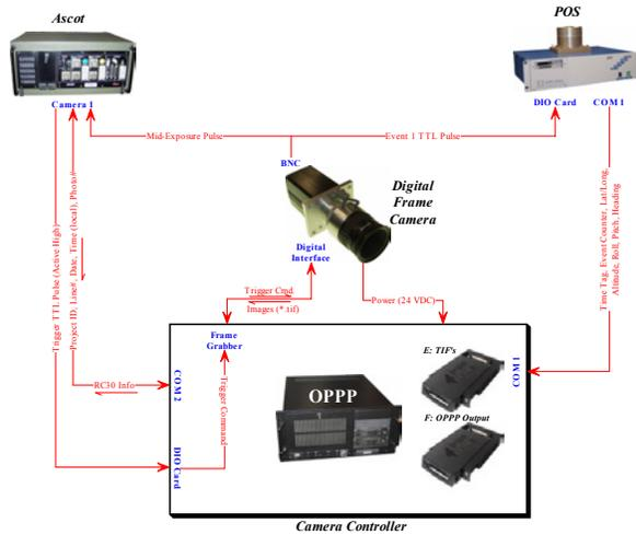
Figure 4. Hardware integration of the OPPP with the DFC, POS, and ASCOT.
