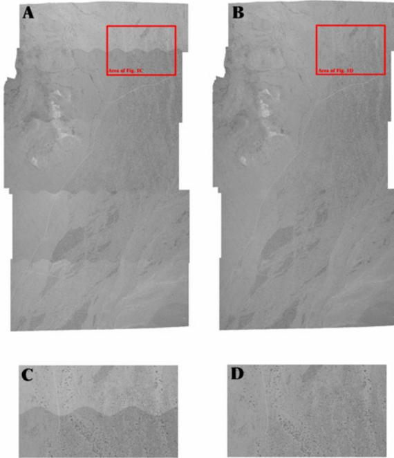
Figure 1. Orthophoto mosaic generated by the OPPP software using scanned RC-30 photographs. A & C – Color unbalanced; B & D – Color balanced.
