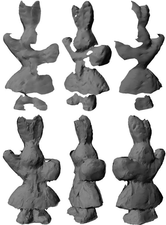
Figure 1: First row contains three 2.5D views of the bunny. The second row contains the complete 3D model viewed from different angles.
