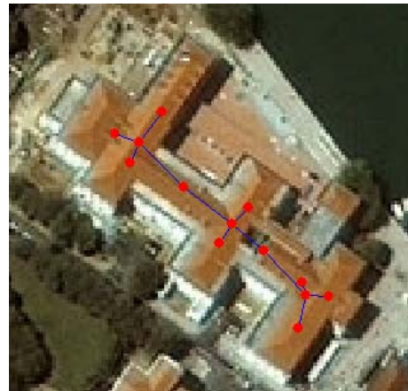
Figure 4. Detecting building structure (Singapore) in IKONOS image – an intermediate state with 13 neuron graph
