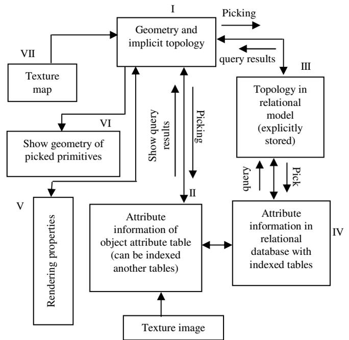
Figure 3. General representation of geometry and topology
