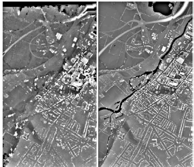
Figure 7: Left, feature layer created from 1:10,000 photogrammetry DSM; right, feature layer created from LiDAR DSM. Both images used a Fourier transform Gaussian low pass filter.
