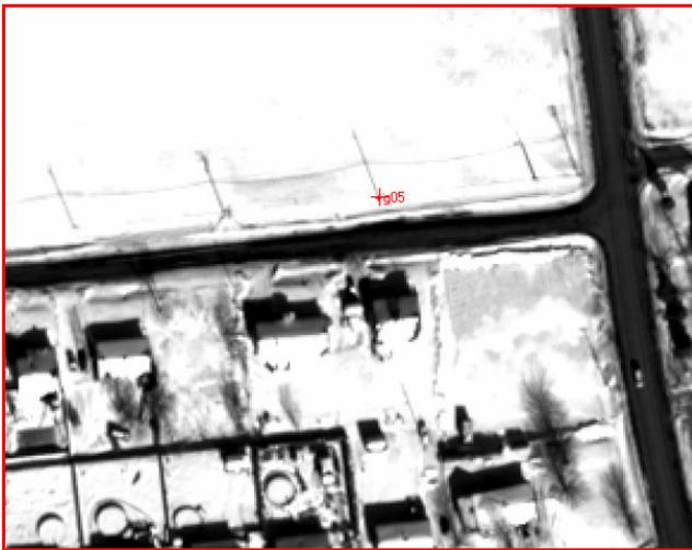
Figure 3. Example of GCP collected with hand-held GPS: the pole defined with its shadow. Even the shadow of the power line is visible on the snow.
