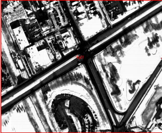
Figure 2. Example of GCP collected with topographic map: the road intersection.
