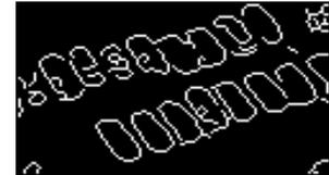
Figure 9. Canny edge detection results of left image
