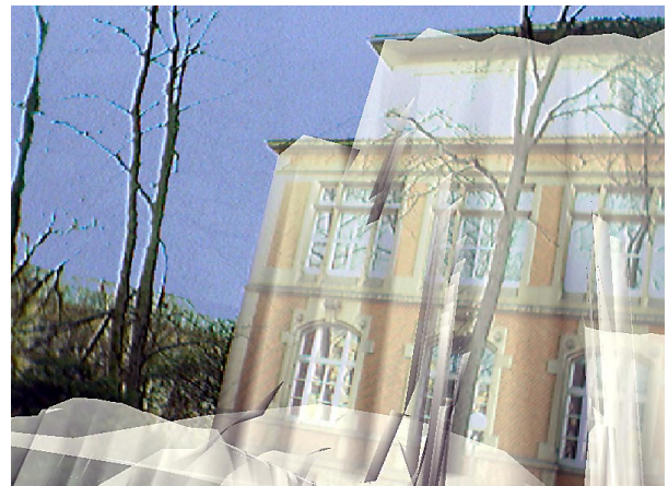
Figure 6. Superposition of video and laser-scanning model
