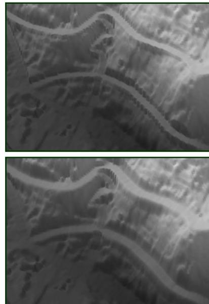
Figure 2: Section from the DTM Stuttgart; resolution 1 m; top: streets broadened around middle axes, bottom: bordering regions adjusted with linear interpolation within a given buffer zone.
