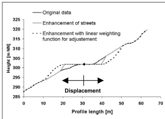
Figure 3: Cross section
