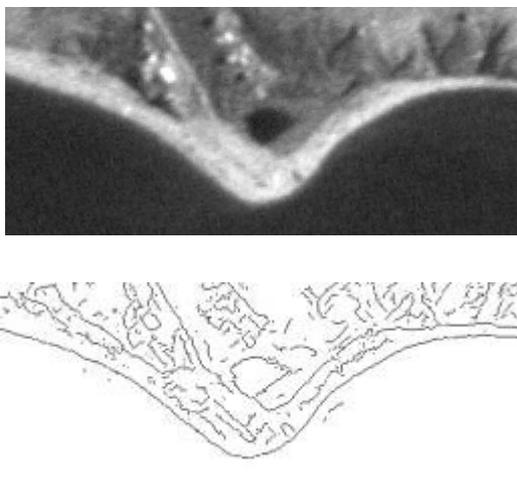
Figure 7: Extraction of coastline using the Canny edge detector.
