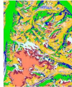
Figure 2: ISODATA clustering using Landsat 7 bands 4,5,7.
