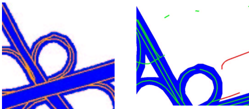
Figure 4: Road network matching; left: detected polygons in orange, dilated and filled polygon in blue; right: polygonal match. Matched DB elements in green. False detected elements in red.
