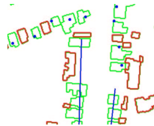
Figure 5: Matching BUA; in blue: detected buildings noted as points and lines; in green: matched DB buildings; in red: missed DB buildings
