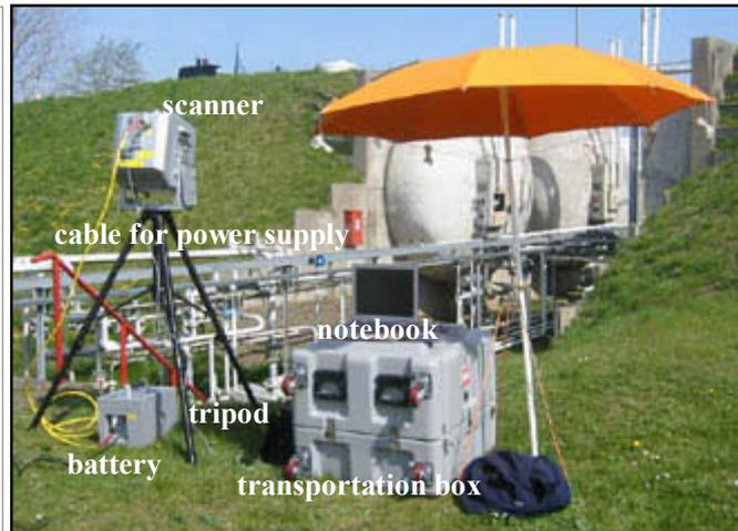
Figure 4. 3D Laser Scanning System CYRAX 2500 at Boie Lübeck
