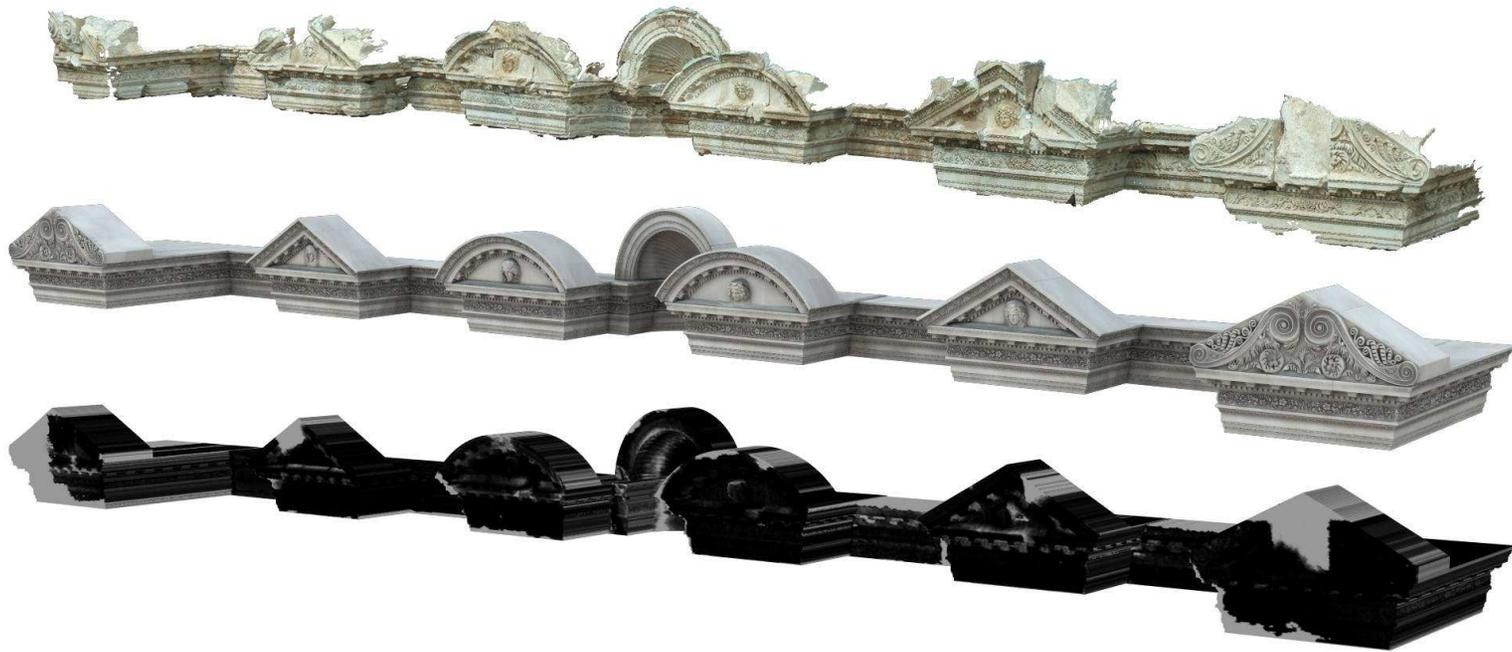
Figure 9: Comparison of captured 3D data (top) and the reconstructed model (middle) for the aediculae. High intensities in the bottom figure correspond to large differences between these two and hence large uncertainties.
