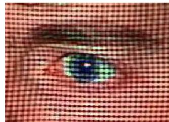
Figure 4: Top: The ShapeCam system consists of a flash projecting a grid and a camera. The camera takes an image from a direction that is slightly different from the direction of projection. Bottom: A regular square pattern is projected on the scene, as seen in this detailed view. 3D co-ordinates are calculated for all the line intersections, resulting in the simultaneous measurement for thousands of points.
