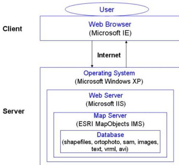
Figure 4: Architecture of web-based multimedia GIS application.
