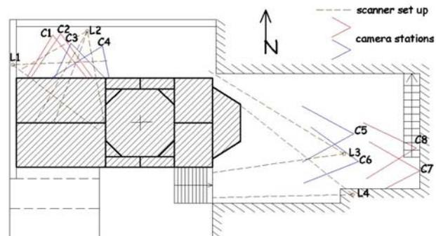
Figure 2. Plan view of the church, showing scanner set ups and camera positions (not to scale)
