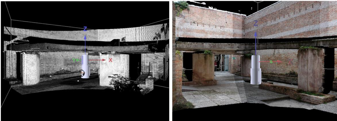
fig. 2 Point clouds union. In the second image points are colored by RGB data acquired with calibrated digital camera
