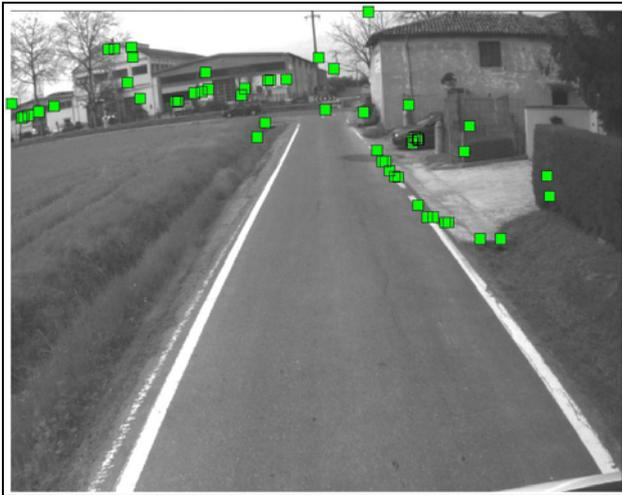
Figure 4. Ground points distribution after the trifocal tensor filtering. Grass presence on the image left area prevents any reliable matching to be found.
