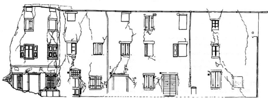
Photogrammetrically plotted cracks after the earth quake in Friuli (1976)
