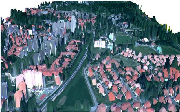
Figure 2. 4 meter DEM instead of real 3D objects
