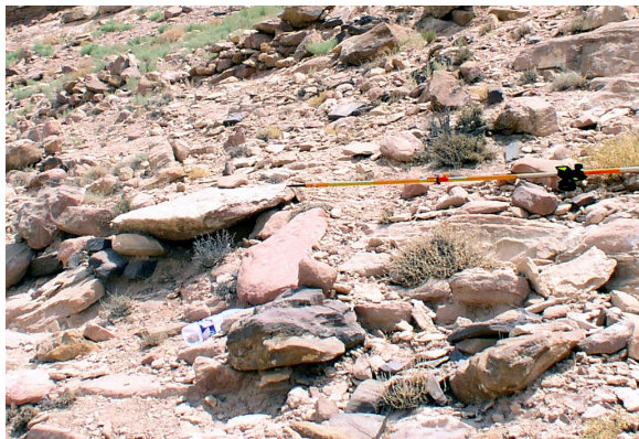
Figure 10. Point No. 24 (Fig. 9) photographed for photogrammetric identification. The exact location is shown here by a measuring stake. It is essential that the viewing direction be close to the same than the one of survey images (Fig. 5).
