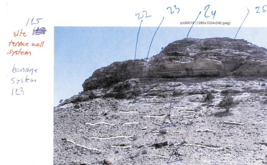
Figure 7. Since no targeted control points are used, recognition of natural features becomes essential part of the fieldwork of photogrammetric documentation. Proper candidates are marked here with triangles. The remains of structures are identified during archaeological survey and marked on prints (here shown in white).
