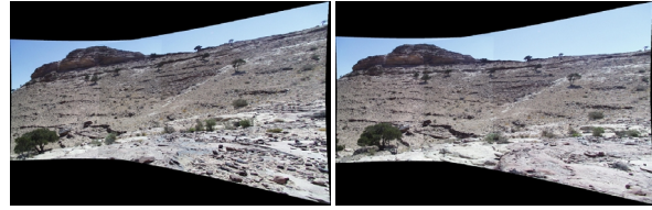
Figure 5. Survey images are based on concentric image sequences. The images are transformed to the normal case of stereoscopy and rectified on planes. The structures are measured from stereo images. The angle of view of this panoramic composition corresponds to 92° x 67° horizontally and vertically.
