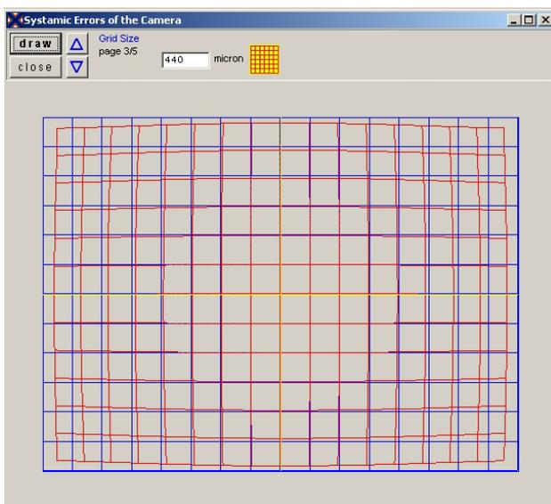
Figure 5. Distortion of wide-angle status (red: current distorted image, blue: ideal undistorted image)
