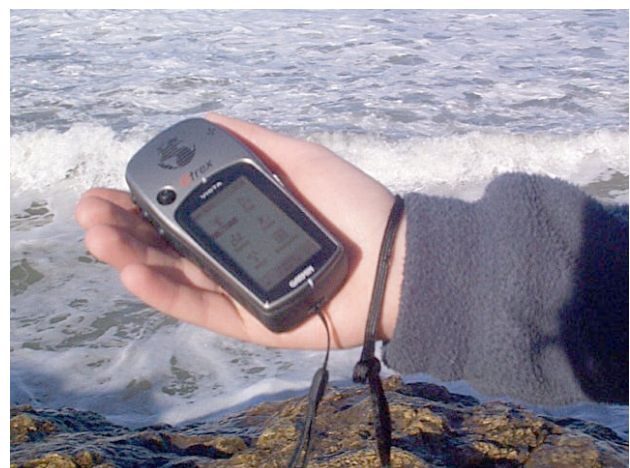
Figure 6. A handheld GPS receiver used in a coastal survey
