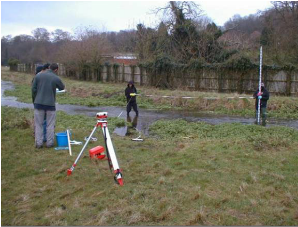
Figure 7. River survey conducted using an engineering level
