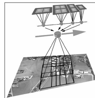
Figure 2. Explaining the difference between „synchronous“ and „syntopic“ image acquisition. The synchronous mode triggers all 4 separate cones at the same time. The syntopic mode triggers them at an interval defined by the flight velocity, about 1 msec apart. © Vexcel Imaging Austria, Copyright 2003
