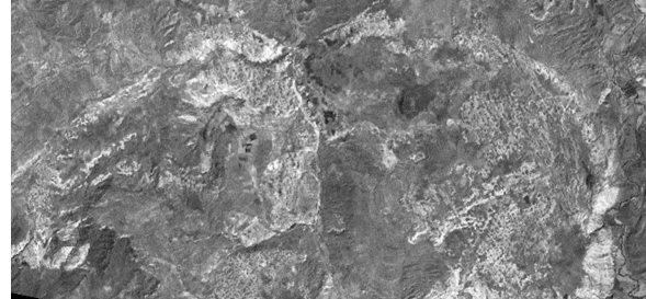
Figure 2: Décollement gypsum levels on band 5, Landsat ETM+ image are highlighted in white.
