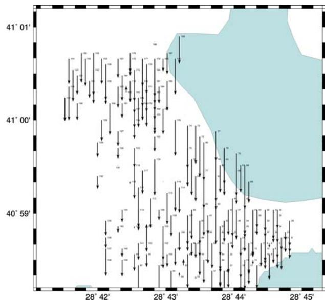
Figure 8. Displacement vectors for vertical coordinates between the years 1999 and 1987
