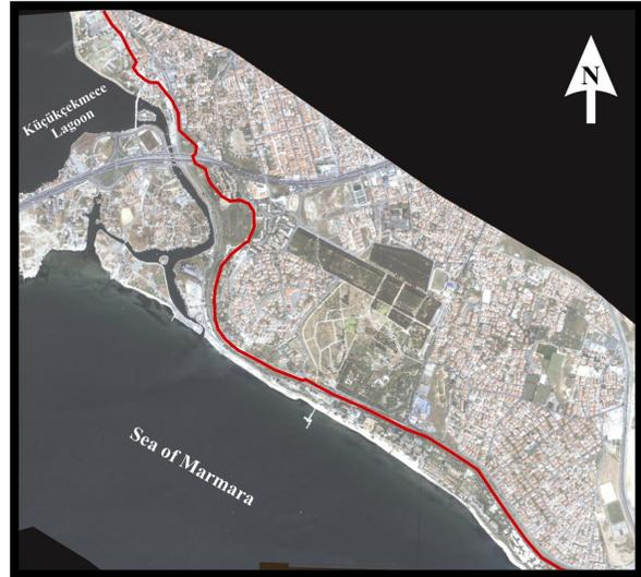
Figure 1. Inundation map drawn for the coastal area in front of Küçükçekmece lagoon. The line shows how far inland and uphill a tsunami caused by an underwater failure is expected to go. Taking into consideration the simulated tsunami waves due to scenario underwater failures, topographic elevations, settlement conditions and geographic characteristics of the inundation area, the maximum inland flooding limits were developed for the wave heights of 2 m at shore.
