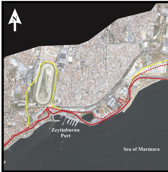
Figure 3. Inundation map drawn for the coastal area in front of Zeytinburnu port. Line definitions are same as in Figure 2. The inundation distance was calculated on the basis of circumstantial characteristics of the inundation area along the coastal zone which was classified for smooth terrains and areas covered in buildings.
