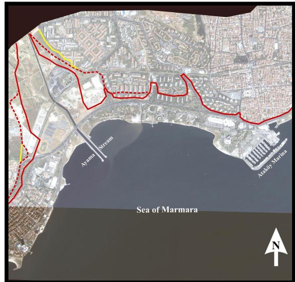
Figure 2. Inundation map drawn for the coastal area of Yesilkoy airport, Ayamama creek and Ataköy Marina. Each line shows how far inland and uphill a tsunami caused by an underwater failure is expected to go. Taking into consideration the simulated tsunami waves, the maximum inland flooding limits were developed for the wave heights of 2, 2.5 and 3.0 m at shore, respectively.
