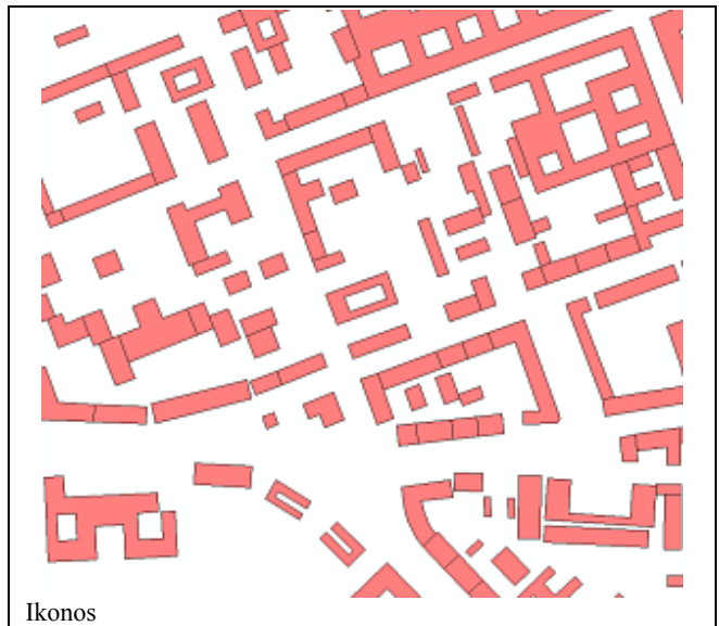
Figure 2. Fragments of vector maps with a layer of „buildings”, scale some 1:5 000 (marks: TBD – contents of the complete TBD data base, ORTO, QB, IKONOS, EROS – results of vectorisation respectively on aerial photographs 1:26 000, and images: QuickBird, Ikonos, EROS)
