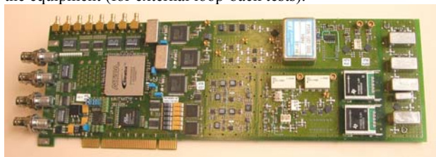
Figure 7. Test Modulator board
