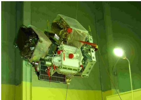
Figure 7: TopSat (on left) mounted on the launch adaptor with ride share partners
