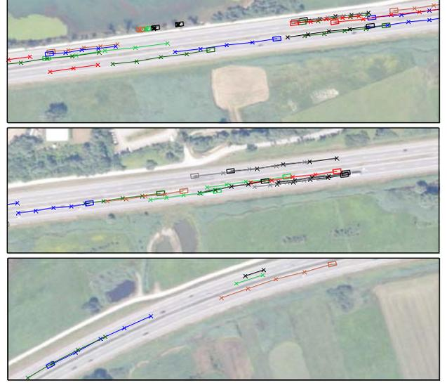
Figure 9. Results of tracking over 5 images. Preceding positions are marked by a cross, the current (last) position is marked by the rectangle. The images show only small sections of the entire picture.
