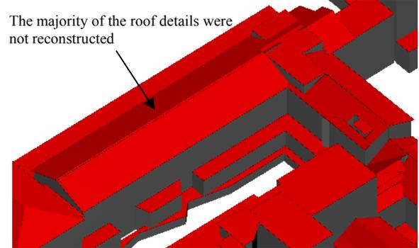
Reconstructed Building from single path LiDAR (2 p/sq.m density)
