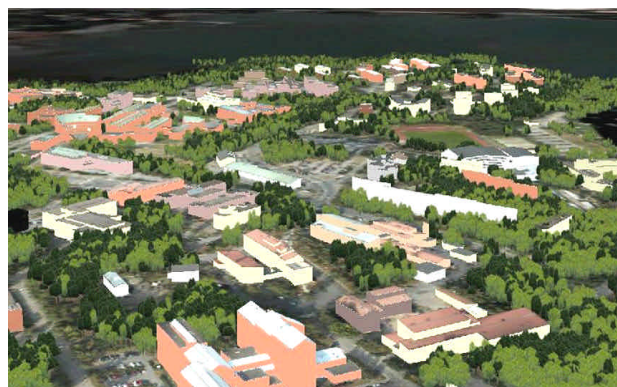
Figure 4. Tree instances generated from the SPOT satellite image 2005 and integrated to Otaniemi city model. ©Terrasolid 2001, © VTT 2006.
