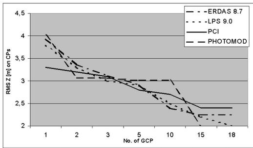
Figure 6. Cumulative diagram of comparative results for generation of DSM depending on a number of GCP with a use of programs ERDAS, LPS, PCI and Photomod
