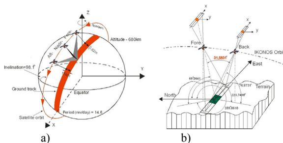
Figure 2. Orbital Geometry (a) and parameters of data along-track IKONOS stereo images (b)
