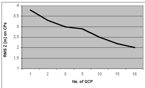
Figure 4. Altitude accuracy (on control points - CPs) for generation of DSM depending on a number of GCP in environment LPS 9.0
