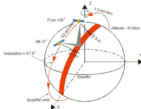
Figure 7. Elements of the orbit of system Cartosat-1.
