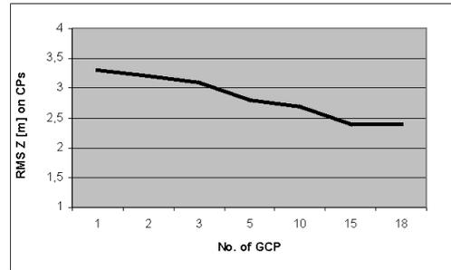
Figure 3. Altitude accuracy (on control points) for generation of DSM depending on a number of GCP in environment PCI Geomatica
