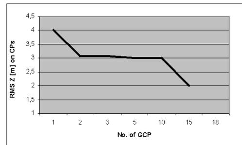
Figure 5. Altitude accuracy (on control points) for generation of DSM depending on a number of GCP in environment Photomod
