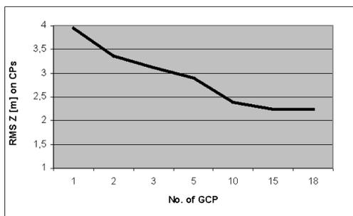
Figure 4. Altitude accuracy (on control points - CPs) for generation of DSM depending on a number of GCP in environment ERDAS 8.7
