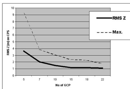
Figure 9. Altitude accuracy (on control points) for generation of DSM depending on a number of GCP with the use of polynomial method (RPF) in environment PCI
