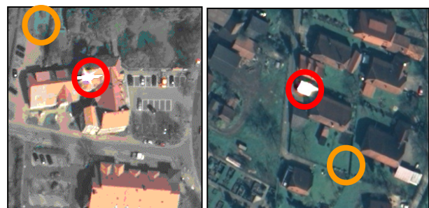
Figure 5. Radiometric effects of total reflection (red circles) and influence of the near infrared on the blue channel (orange circles), flight for Land Survey Department Lower Saxony
