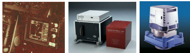
Figure 1. System configuration with flight navigation system CCNS4 (IGI), GPS/INS (IGI), DMC (Intergraph)
